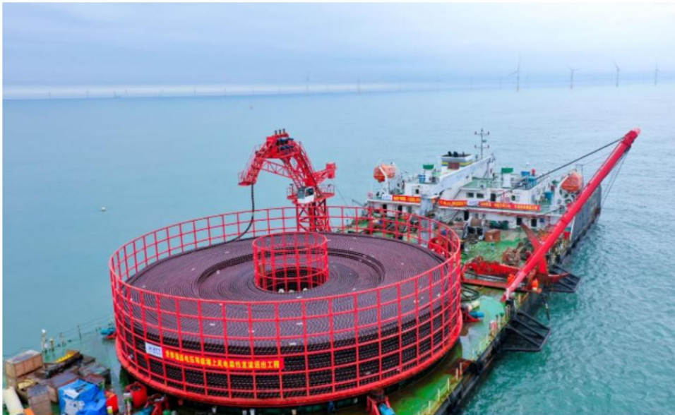
Figure 3-1: The smooth delivery and operation of the \pm 400 kV DC submarine cable contracted and laid by Zhongtian Technology
